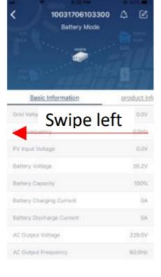
Basic Information displays basic information of the inverter, including AC voltage, AC frequency, PV input voltage, Battery voltage, Battery capacity, Charging current, Output voltage, Output frequency, Output apparent power, Output active power and Load percent. Please slide up to see more basic information.
