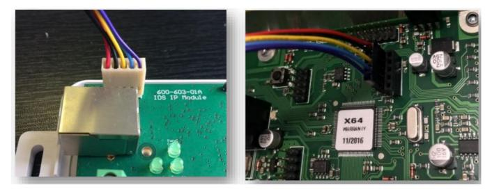
Plug in the Ethernet cable from the network to the Ethernet connector, or connect to your WiFi. If the WiFi module is installed the Ethernet port is ignored.
