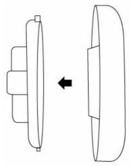
4. Then, attach the mounting screw to the back of the adapter (the Nest Cam base is magnetic, so the mounting screw will line up easily with the adapter hole). Twist the Nest Cam base clockwise until it's firmly in place.
