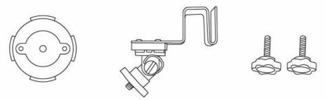
2. Attach the mounting piece by first taking out the screw at the base of the gutter mount and sliding the mounting piece in between the slots. Then, put the screw back in and tighten it firmly.
