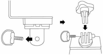
3. Attach the Nest Cam adapter to the bottom of the Nest Cam base by lining up the flanges and twisting until the adapter locks into place.
