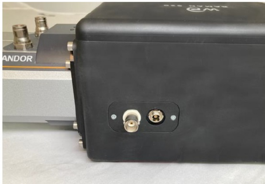
Spectrometer shutter connectors (cable, left; power, right)
