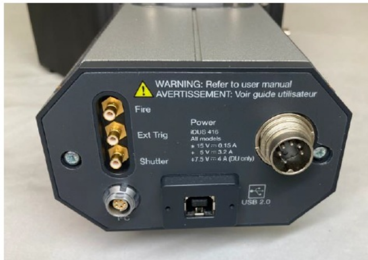
Andor camera connectors (shutter, left; power, right; USB, bottom)
