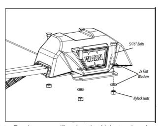
5. Installation of bracket complete. Read your specific relocation kit instructions for complete relocation instructions.
