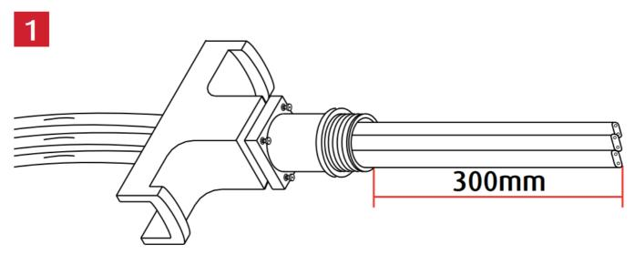
Push the heating cable(s) through the lower bracket, leaving 300mm of heating cable exposed. **NOTE:** Max. 3 heating cables.
