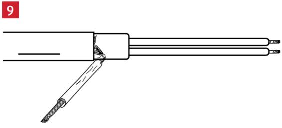
Insert the bus wires through heat shrink tubes. Insert the braiding through the ground tube.
