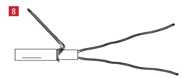
Cut the exposed self-regulating matrix back to the heating cable insulation. DO NOT CUT THE BUS WIRES.
