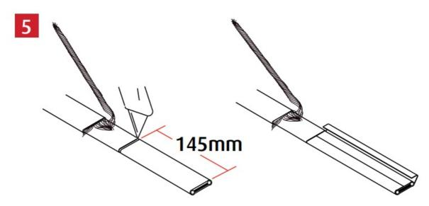
Separate the bus wires from the self-regulating matrix material with a utility knife.
