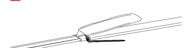
Peel back the exposed bus wires. DO NOT CUT THE BUS WIRES.
