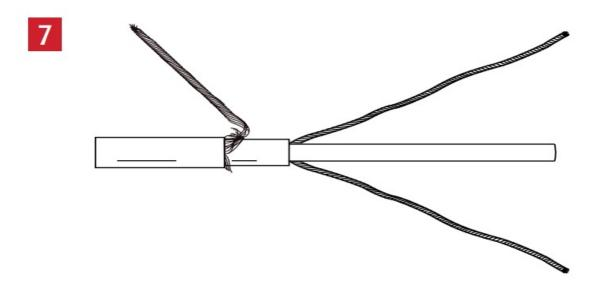
Cut the exposed self-regulating matrix back to the heating cable insulation. DO NOT CUT THE BUS WIRES.
