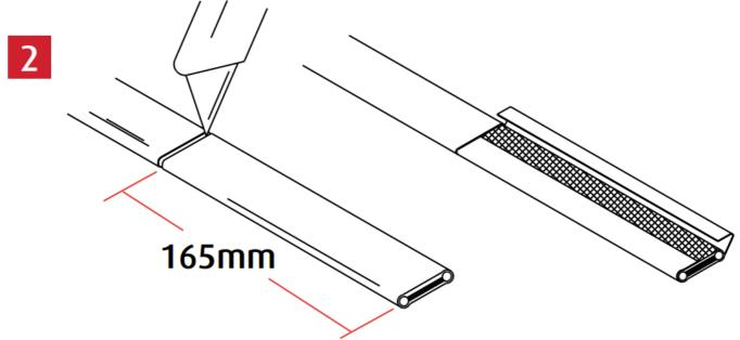
Measure 165mm in from the end of the cable and carefully cut the outer sheath. Bend the cable to break sheath. Next, gently slice the outer sheath up the centre between the first cut mark and the end of cable. Bend the cable to break sheath and remove the sheath from the heating cable.
