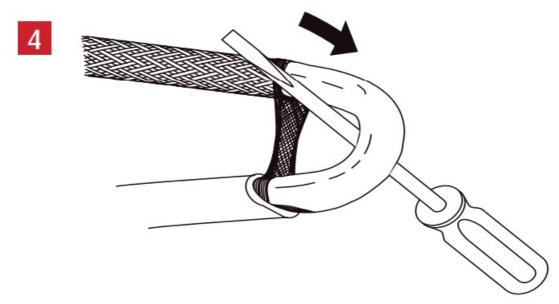
While bending the heating cable, work the heating cable through the braid opening and then pull the braid tight and twist.
