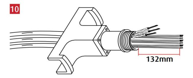
Insert the prepared cables into the lower bracket ensuring they extend 132mm beyond the bracket, and then tighten the 4 screws.
