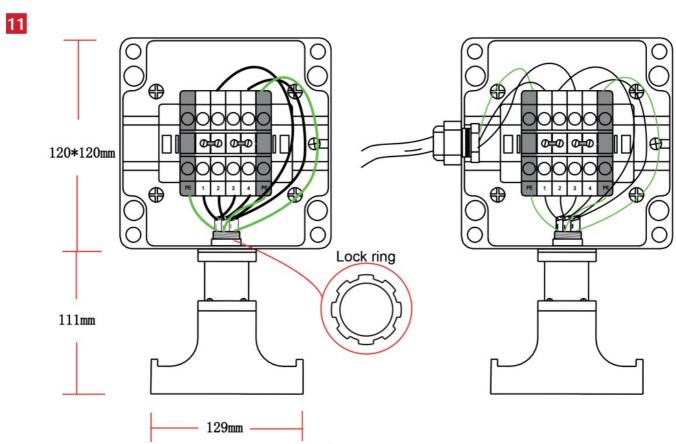
Insert the cables through the base of the junction box. Secure the lower bracket to the junction box using the lock ring.
