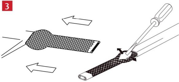
Move the braid back toward the outer sheath. At the base of the braid where it meets the outer sheath, gently
