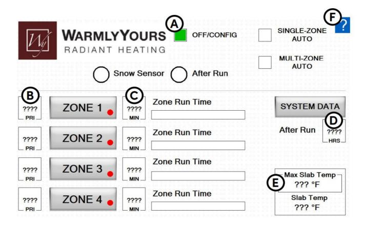
Pri this is where the user can determine the run order of the zones 1-4. Note- the system will not allow for more
