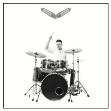
• In this diagram, two WA-87 R2s are used in a coincident pair, also known as XY configuration, to record stereo drum overheads.
