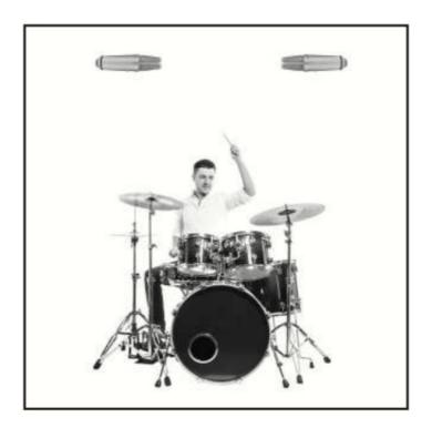
• In this diagram, two WA-87 R2s are used in a spaced pair configuration to record stereo drum overheads, maintaining an equal distance from the snare drum for proper phase.
