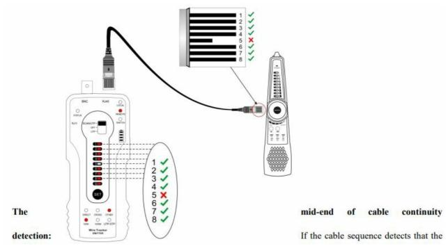
• cores of the cable are disconnected, and the local/remote cores are detected to be connected, indicating that the break point of the cable is in the middle position away from the ports on both sides.
