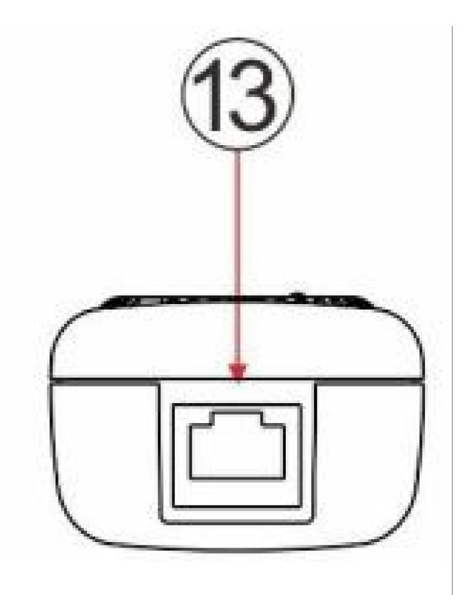
Note: Receiver port continuity detection only supports the local end, and does not support the remote end. Emitter can support near-end, middle-end end, and far-end port detection.
