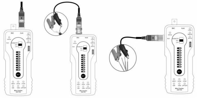
1. Adjust the switch of the emitter to the "Scan/UTP" mode, and press the "SET" key to switch to UTP/STP mode. The green light of the "UTP/STP" indicator means normal mode, while the red light is shielded mode. Turn on
