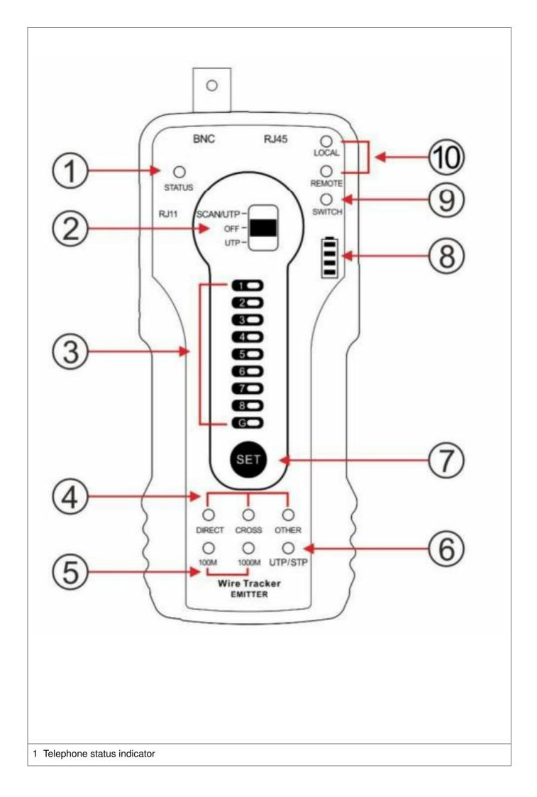
2 Functions switch: SCAN/UTP, OFF, UTP cable test
