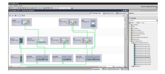
In this example, the Lean Managed Switch with part number 852-1812 was integrated into a test system. To ensure that no errors are displayed in the TIA Portal, monitoring of the ETHERNET connections between the Lean Managed Switch and the other Conformance Class B devices must be deactivated.
