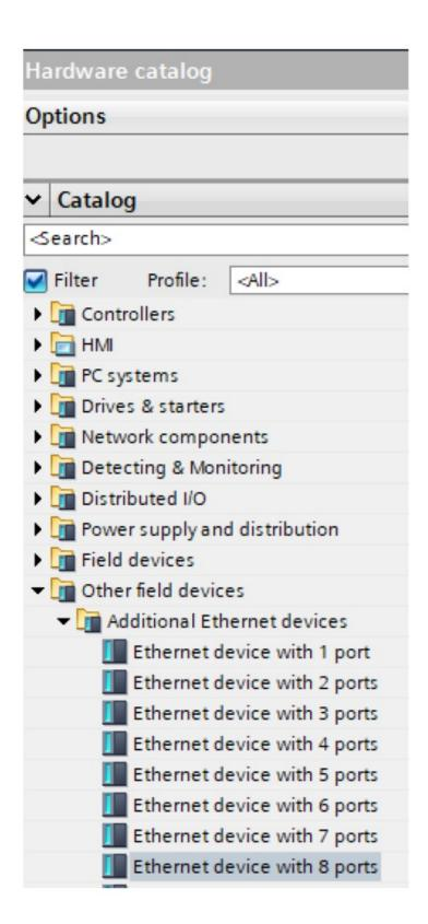
To integrate the product 852-1812 into a PROFINET® project the marked "Ethernet device" from the hardware catalog must be used.
