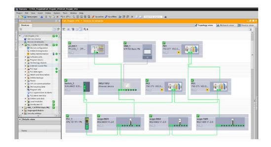
Now the ETHERNET connection between the 0852-1812 and the pfc200-1 has been interrupted. A system error can be recognized directly
