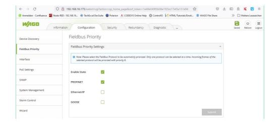
In the default setting, the prioritization of the PROFINET® data packets are enabled. Ethernet/IP and GOOSE data packets can also be prioritized in this menu.
