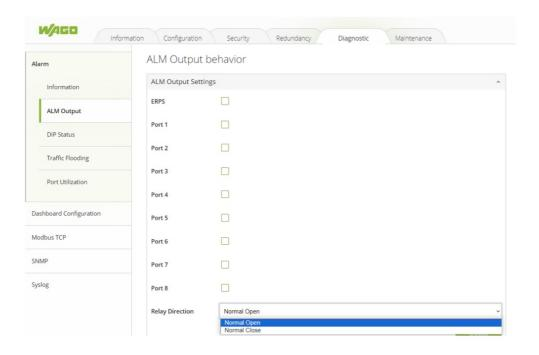
The port parameter indicates the status of the monitored port (port link up or link down). An alarm will occur if there is a port link up or link down. In this case, the ALM relay changes status. The status of the ERPS rings can also be monitored.
