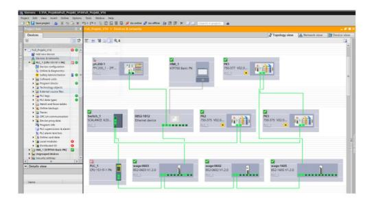
The analysis of the diagnostic buffer clarifies the loss of connection of the PROFINET® device pfc200-1. The PROFINET® device pfc200-1 is not reachable.
