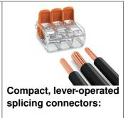
Tool-free connection of fin e-stranded conductors fro m 0.14 ... 4 mm², as well as solid or stranded conductors from 0.2 ... 4 mm² (24 ... 12 AWG).
