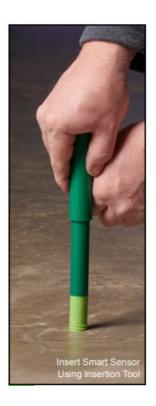
**TIP:** Check the L6 Smart Sensor prior to installation to ensure there is a properly functioning sensor that is giving a reading.
