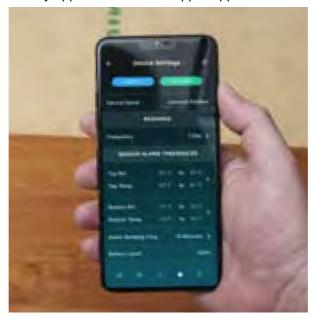
• Step 3. Open the app, give your Floor Sentry device its unique name, adjust the default settings (as needed), click the Device Installed button on the Device Settings screen, and you are ready to begin monitoring temperature and RH at whatever frequency you desire.
