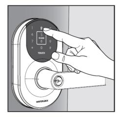
• Step 3Press 7#, there will be 2 short beep sounds. Key in 001#, there will be a long beep sound, meaning the passcode anti-peeping mode is OFF. Key in 002#, there will be a long beep sound, meaning the passcode anti-peeping mode is ON.
