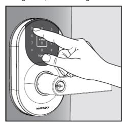
• Step 3 Press the "TOUCH" key, the keypad lights up, and then press \*\*\* #. A long beep sound and blue light will blink 5 times to successfully remove all user credentials.
