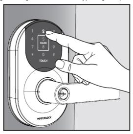
• Step 3Press \*\*\*#. A long beep sound and blue light will blink 5 times to successfully remove all passcodes.
