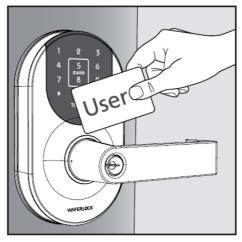
• Step 2 The keypad LED runs clockwise when access is granted
