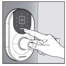
• Step 2Key in the 6-digit passcode and press #, the LED will run clockwise when access is granted.
