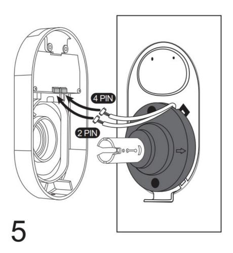
1. Well connect the cables to the connectors of inside assembly.
