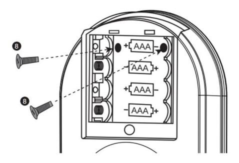
1. Tighten the fixing screws at the battery box of the inner unit.
