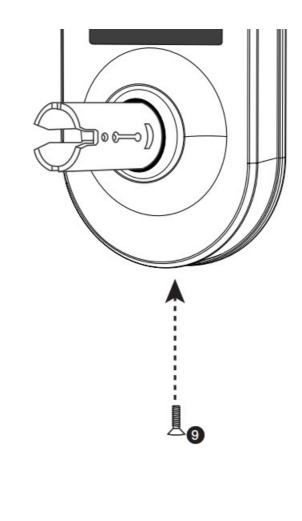
1. Install insdie assembly and tighten the fixing screw from the bottom.
