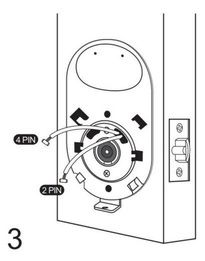
1. Take the backplate, gently thread the cables from the outside assembly through the hole located near the latch in the backplate.
