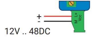
The switch is ready for standard operation after a few seconds.
