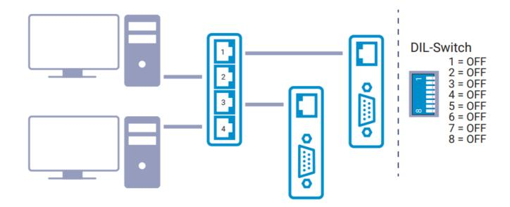
Each port automatically detects the transmission rate and whether data transmission should be in full or half duplex mode.
