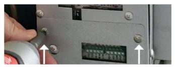
3. Using a precision screwdriver, change the Dip Switches positions for S3 (Up/On) and S9 (Dn/Off) to enable Wall Thermostat control.
