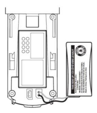
2. Place the battery with the label THIS SIDE UP facing up and the wires inside the battery compartment.
