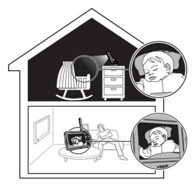
The baby unit has infrared LEDs that allow you to see your baby clearly at night or in a dark room. When the baby unit being viewed detects low light levels, the infrared LEDs are switched on automatically. The images from the baby unit are in black and white, and cappears on the screen.
