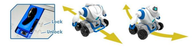
• Switch the Steering Lock Switch to the Unlock position to enable steering variations. IMPORTANT NOTE: the Steering Lock Switch should be locked for the missions to work as intended.
