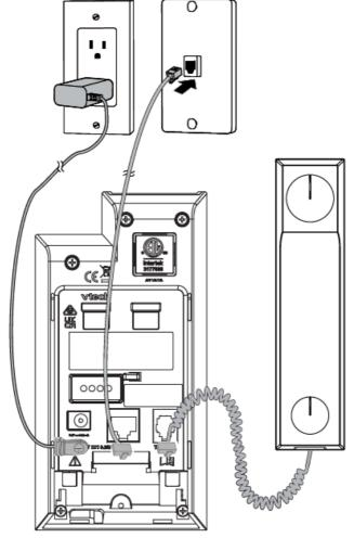
If you are connecting a power adapter, make sure it is securely plugged into an outlet not controlled by a wall switch, and the ethernet cable is plugged into the network wall jack.
