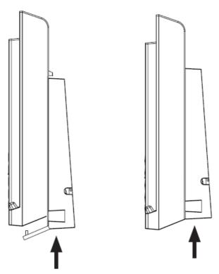
Connect the telephone as described in "Telephone base installation" on page 10, but use the short ethernet cable.
