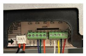
5. Plug the VTech Wiring Harness into the Controller module. Press the connector firmly to ensure it snaps into place securely. Then, restore power to the PTAC/PTHP.
