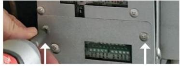
3. Using a precision screwdriver, change the Dip Switches positions for S3 (Up/On) and S9 (Dn/Off) to enable Wall Thermostat control. Note: Switch labels are located on the PCB, just below the switch assembly.
