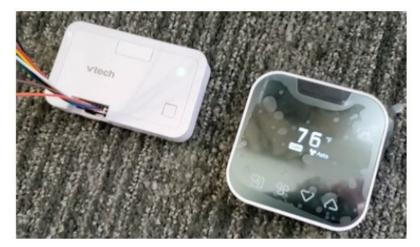
10. Mount the controller to the PTAC chasse and secure wiring. Cover/protect unused wire leads. Route the wires so they do not sag into the condensation pan.
