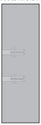
3. Align the wall mount bracket and screws with the holes in the wall as shown. Tighten the screw in the middle hole first, so that the wall mount bracket position is fixed. You can tighten the other screw in the top hole.
