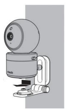
5. You can maximize your camera unit's viewing angles by tilting the wall mount bracket. Hold the camera unit, and then rotate the knob in anticlockwise direction. This will loosen the joint of the wall mount bracket. Tilt your camera unit up or down to adjust to your preferred angle. Then, rotate the knob in clockwise direction to tighten the joint and secure the angle.
