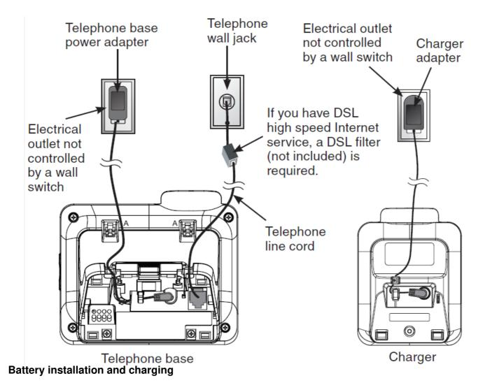
Install the battery as shown below. Once you have installed the battery, you may be able to make and receive short calls. For best performance, charge the handset battery continuously for at least 10 hours
