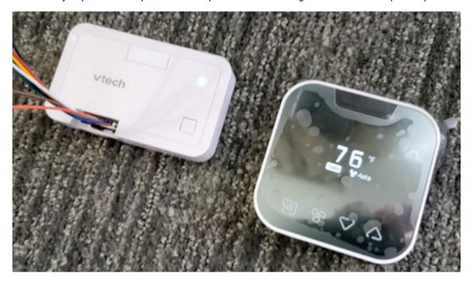
10. Mount the controller to the PTAC chasse and secure the wiring. Cover/protect unused wire leads. Route the wires so they do not sag into the condensation pan. Finally, replace the cover to the unit.
