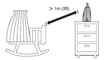
2. Place the parent unit more than 3 feet (1 meter) away from the baby unit to avoid screeching noise.
