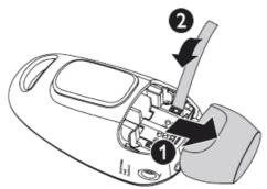
1. Slide open the battery compartment cover.
