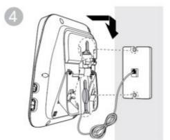
Align and mount the bracket to the telephone wall mount plate.
