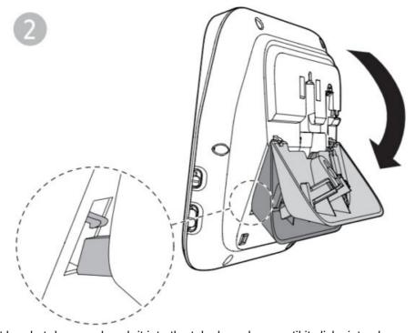
Flip the wall-mount bracket down and push it into the telephone base until it clicks into place.
