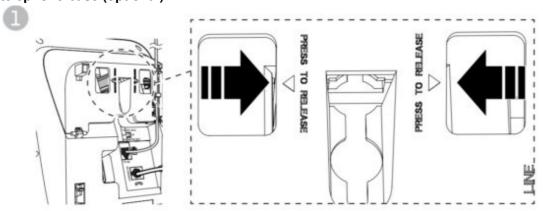
On the rear side of the telephone base, press the tabs of the wall-mount bracket to release it from the tabletop orientation.
