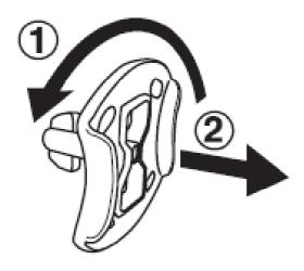
Rotate the packaging locks counterclockwise 90 degrees. Pull out the packaging locks and discard.
