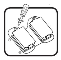
5. Replace the battery covers and tighten the screws to secure.
