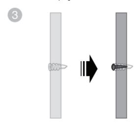
Insert the screws into the holes and tighten the screws until only 1/4 inch of the screws are exposed.
