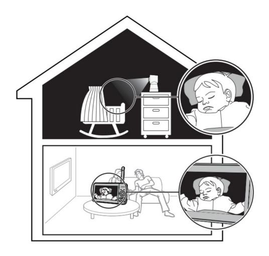
The baby unit has infrared LEDs that allow you to see your baby clearly at night or in a dark room. When the baby unit being viewed detects low light levels, the infrared LEDs are switched on automatically. The images from the baby unit are in black and white, and prears on the screen.
