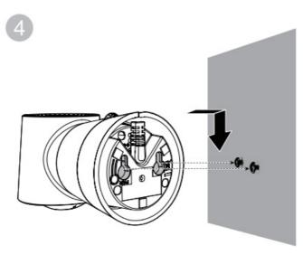
Align the wall mount holes on the baby unit with the screws on the wall. Slide the baby unit down until it locks into place.
