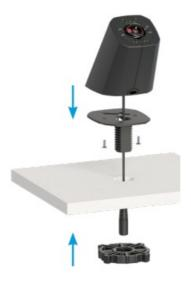
**B.** Place the connected pedestal and adapter through the hole in the fixture and tighten nut.
