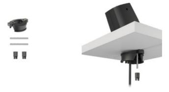
Screw the threaded rods through the mounting ring and into the pedestal. Mount to the fixture with the two thumb nuts. Skip to step 6.
