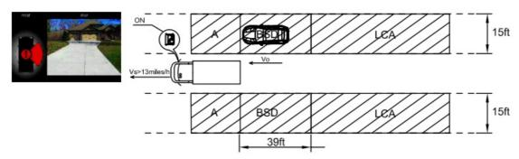
• The warning light will illuminate if there's a slower target vehicle, relative to the moving vehicle's speed, (Vs-Vo<7miles/h) in BSD detection area.
