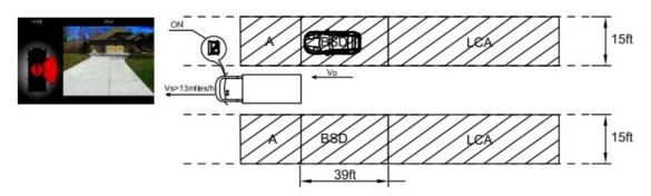
• If an LED is illuminated and it's corresponding turn signal is triggered, the LED will blink and the Buzzer will provide an audible alert/beep.
