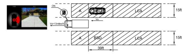
The warning light will illuminate if there's a stationary target vehicle, relative to the moving vehicle's speed, (Vo=Vs) in BSD detection area.
