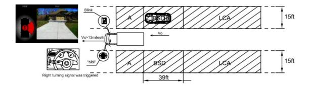
• The warning light will illuminate if the target vehicle in the LCA detection area will overtake the vehicle within 5 seconds.
