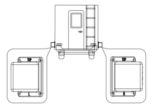
Use 4 screws to affix the Sensor to the vehicle once the correct position is found and use Cable Ties to tie down Harness wiring. Note: Make sure that the Sensor's orientation is parallel to the vehicle's body.
