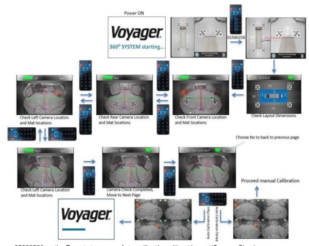
2. Press 85208520 on the Remote to access Auto-calibration without Layout/Camera Check
