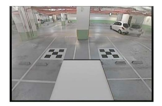
**Note:** Reverse trigger has the top priority. Whenever the turn light and backward are both triggered, the VAVSMOD2 shows the backward view.
