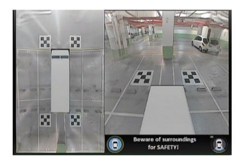
If the Left Turn Signal is triggered, the VAVSMOD2 will give the driver a top view and left-side view
