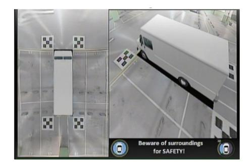
If the Right Turn Signal is triggered, the VAVSMOD2 will give the driver a top view and a Right-side view
