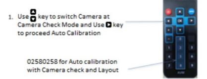
85208520 for Auto Calibration without Camera Check and Layout
