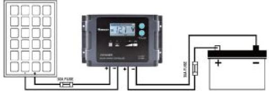
**NOTE** The solar controller should be installed as near the battery as possible to avoid efficiency loss. **NOTE** When the connections are completed correctly, the solar controller will turn on and begin working automatically.
