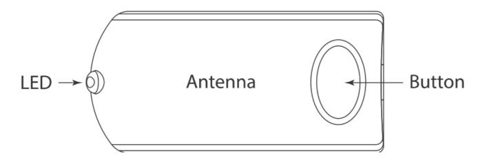
The Control Center sends and receives commands or messages to and from the system. It consists of:
