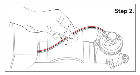
3. Open the compressor cover and note the corresponding (R, S, C) color of the wires.
