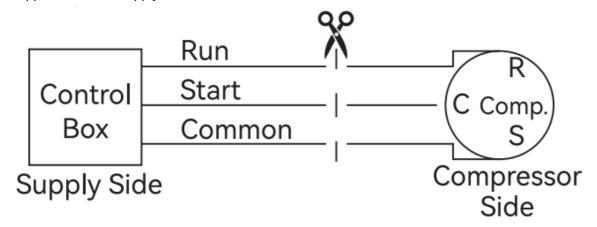
6. On the compressor side, carefully match the cut run, start, and common wires coming from the compressor with the run, start, and common wires on the COMPRESSOR side of the soft starter. Strip each wire by %" and terminate all 3 connections using closed end splice connectors.
