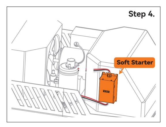
5. Cut the compressor three wires at a location within range of the soft-starter wire harnesses. Clearly identify the supply and compressor sides of the connections. In this illustration, Lower section is Compressor side and Upper section is Supply side.
