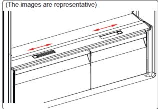
If the crisper is full, the fresh dial located in front of the crisper should be opened. This allows the air in the crisper and the humidity rate to be controlled, to increase the life of food within.
