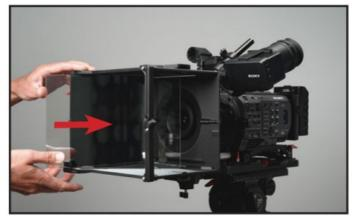
3. The coloured stickers on the beamsplitter glass and main unit must align.
