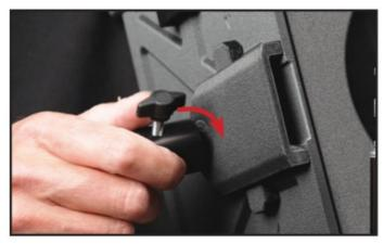
2. Attach the main unit to a light stand and position in front of the lens.
