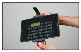
2. Attach the tablet holder to the main unit. There are three locking positions, indicated on the top of the tablet holder.
