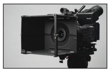
If extra height is needed between the railblock and the lens, it is possible to invert the railblock.
