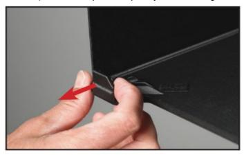
2. Note there are two sides to the beamsplitter glass – observe the coloured sticker which indicates the mirrored surface. Align the glass with the internal rails and slide into the main unit.
