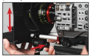
6. – The main unit height should be set as shown. Position the doughnut to create a seal around the opening at the back of the main unit.
