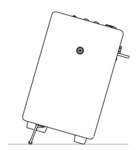
The VOX MINI GO 10/50 can be set at an angle by pulling out two stands at the bottom of the main unit (refer to the figure on the left).
