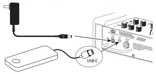
2. Connect the included AC adapter to the DC19V jack (DC 12V jack for VOX MINI GO 3/10) on the rear panel (26), then plug the adapter into an AC outlet.
