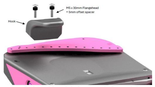
The plate mounts to the footpad through the bumper and rail corner bolts on both the XR and GT frame (XR Pictured). The bolts used to mount the plate are simply extended over the stock size by approximately 8/10mm depending on the frame and plate type. Blocks mounts in the same way as the crossbar, using 30mm M5 flangeheads with 5mm spacers.
