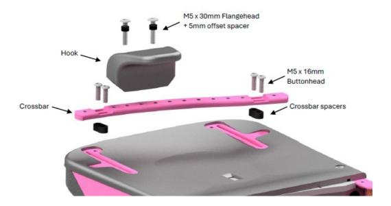
The Crossbar mounts to the Nyloc nuts inside the bolt tracks using the appropriate spacers and 16mm buttonhead M5 bolts. Blocks can then be bolted to the Crossbar using 30mm flange head M5 bolts with 5mm spacers
