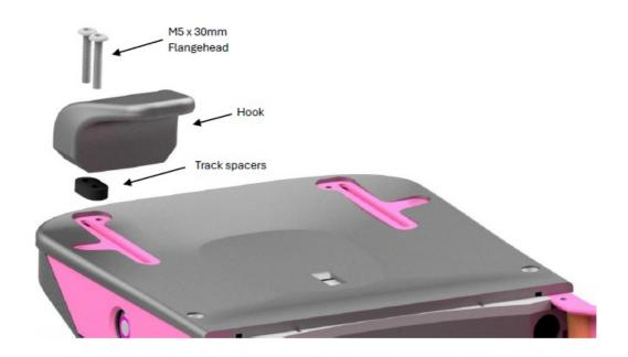
The blocks can be mounted to the bolt tracks individually using the appropriate bolts and spacers. Simply place the block in the appropriate position and tighten the bolts 'fingertight' with a manual screwdriver, not using much leverage. The blocks shouldn't be able to move if the system is correctly tightened. Overtightening can damage the elevon blocks / bolt tracks
