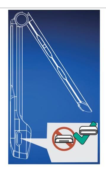
Insert USB cable and charge for 3 hours
