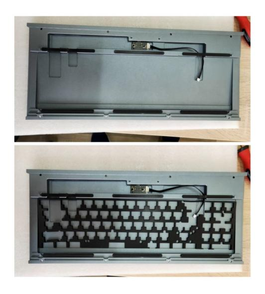
Connect the main PCB with the daughterboard and attach the ffc to the F-row. Place the top case and secure it with M2 black screw\* 8 pcs to complete the assembly.
