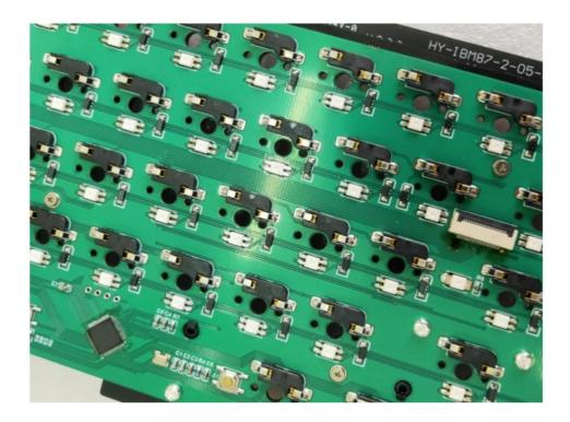
Flip the top case of the kit to the back and position the Poron plate foam, followed by the Poron switch pad along the F-row. Finally, place the PCB on top. Then screin the M2 black screw\*4 pcs.
