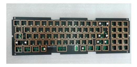
After positioning the mounting plate, flip it over to the backside of the PCB, and secure the previously installed brass standoffs by fastening them with screw
