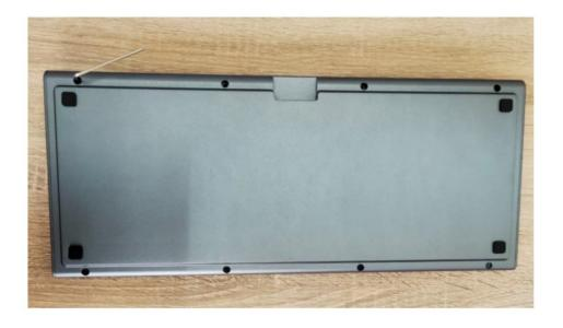
After disassembling the top and bottom case, secure the daughterboard at the marked locations in the picture below, and attach the gaskets according to preference.
