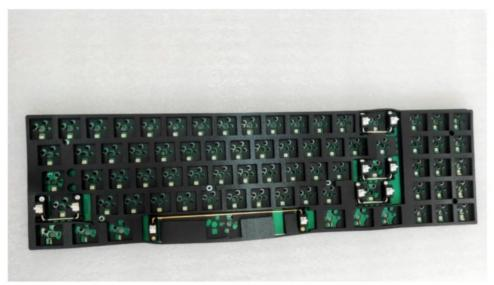
Place the mounting plate (FR-4/brass/aluminum) on top of the Poron plate foam.
