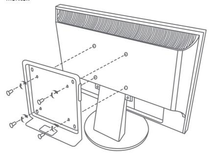
Screw Specification M4 x8L (K)W-ZN #2 Rack size 194 x 150 x 25 mm
