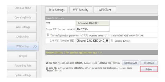
Remark 3: After VONETS device sets the WAN port to access the WiFi hotspot in the routing mode, its LAN port IP is still 192.168.254.254, and the terminal device also obtains the IP address of the same network segment, can login configuration page by 192.168.254.254 or <a href="http://vonets.cfg">http://vonets.cfg</a>.
