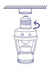
The product adopts a good sensitivity detector and integrated circuit. It gathers automatism, convenience safe, saving-energy and practical functions. It utilizes the infrared energy from humans as the control-signal source, it can start the load at once when one enters the detection field. It can identify day and night automatically. It is easy to install and used widely.
