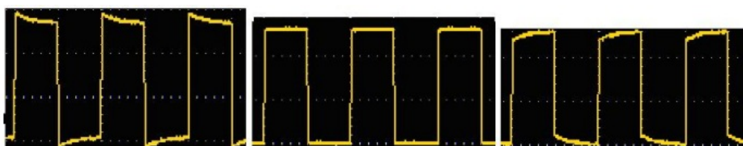
Overcompensated Compensated correctly Under compensated
