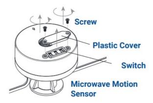
Using a screwdriver, remove the plastic cover from the switch on top of the sensor.
