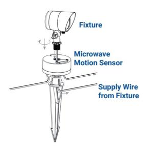
Pass the supply wire from the fixture through the microwave motion sensor with the stake. Thread the fixture onto the top center of the sensor.
