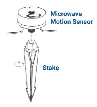
Thread the stake on to the bottom center of the microwave motion sensor.
