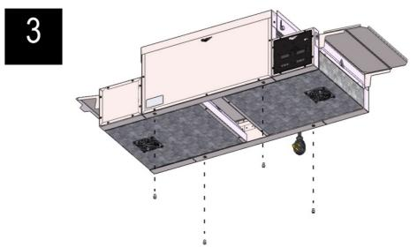
**Note**: The screws help stabilize the top oven, but they do not attach the oven to the stacker.
