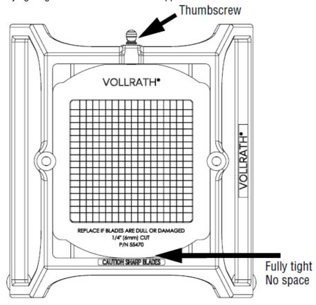
6. Check for proper blade alignment by slowly setting the pusher head on the blade assembly.
