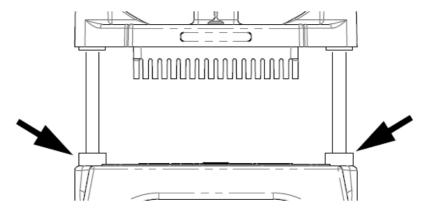
5. Verify the blade assembly is properly installed in the base. The thumbscrew must be fully tightened and the blade assembly fully tight against the side of the frame opposite the thumbscrew.
