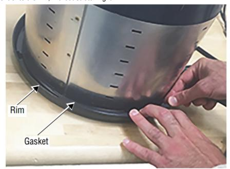
5. If needed, use a scissors to trim the gasket to the proper length.
